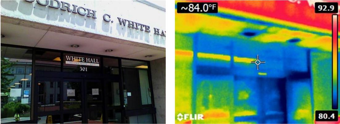
Figure 4 – Exterior image showing leakage at curtain wall and soffit lighting
