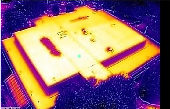
Figure 5 – Thermal imaging of the classroom building roof utilizing drone technology
